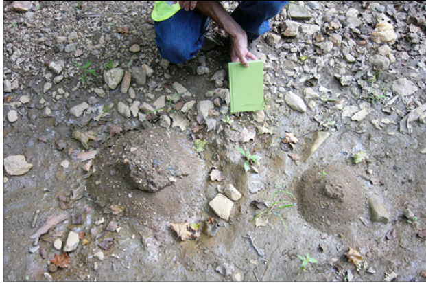
Figure 25. Sand boils near the 2011 Earthquake epicenter. Photo by Mark Carter, U.S. Geological Survey.
